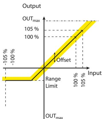
Inverting characteristic with adjustable RangeLimit (max) and adjustable offset
