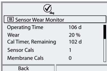
The sensor wear monitor shows the sensor operating time and the maximum temperature during the operating time, as well as wear and the forecast remaining time.
