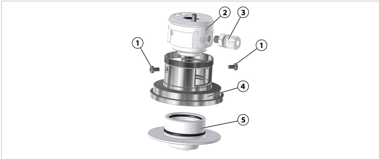
01. Remove the process unit from the drive unit. → *Drive Unit: Removal, p. 36*
